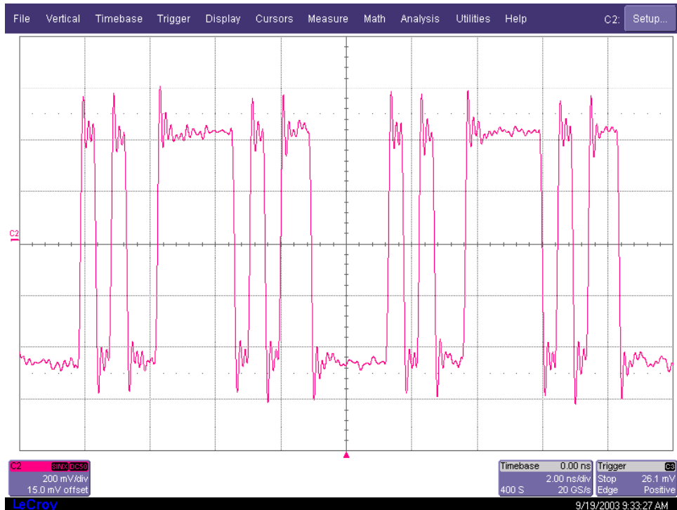
Figure 10 - Lecroy Real Time scope waveform capture of 2.125Gb/s K28.5 pattern.
